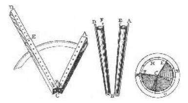
**Figure 2.1.** Comparing and grading lights: Pierre Bouguer's light-measuring apparatus. Left: the lucimètre. Centre: a telescopic version consisting of two equal-length tubes some 2 meters long, one having an adjustable sector aperture (right). The ends of the tubes B, covered with fine white paper, are viewed through a tube to reduce stray light. From Bouguer P 1760 *Optical Treatise on the Gradation of Light* (transl. by W E K Middleton).
