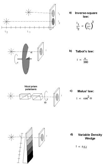
Figure 3.6. Methods used to adjust the reference intensity in visual photometry.
