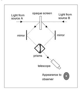
Figure 3.5. Principle of the Lummer-Brodhun photometer head.
