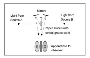
Figure 3.4. Principle of the Bunsen grease-spot photometer head.
